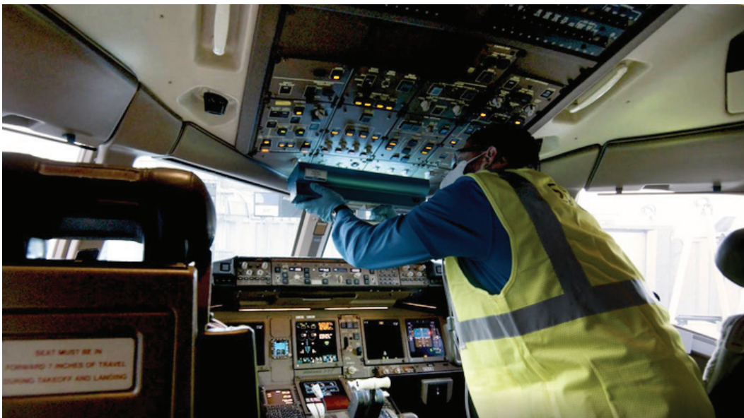
Figure 1. A handheld ultraviolet C-band (UV-C) device to disinfect surfaces [3].
