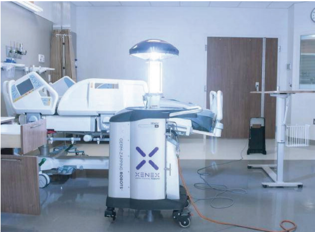
Figure 5. Xenex's disinfecting robot, called LightStrike [8].
